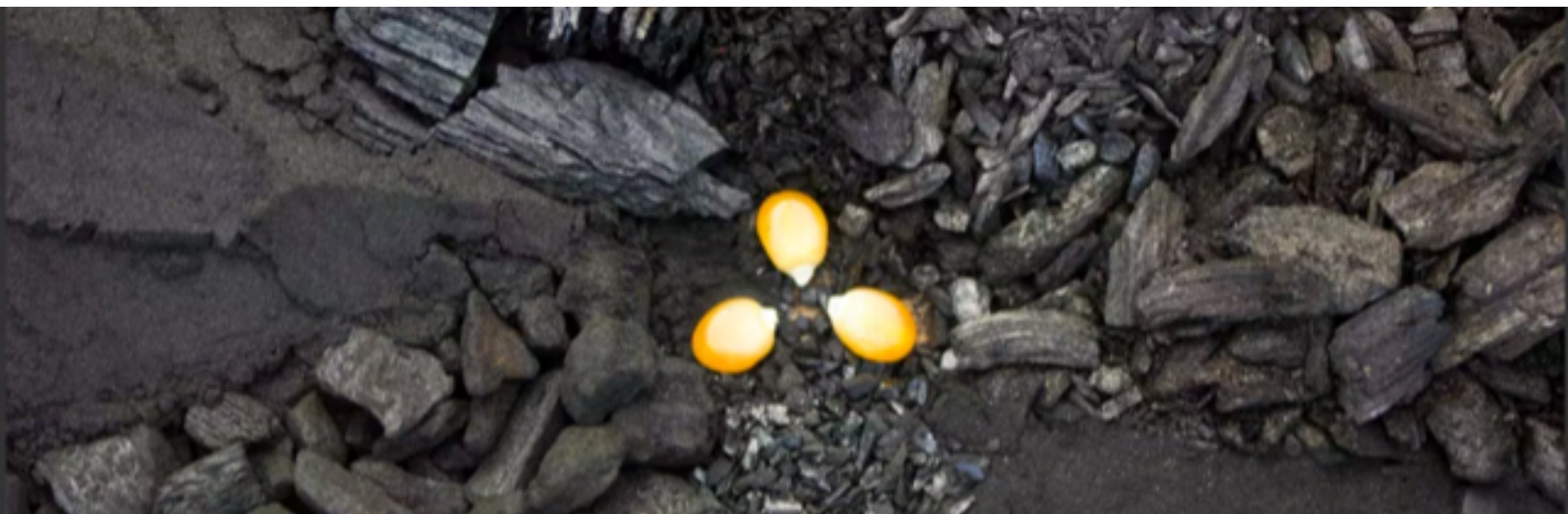
Seven different biochar materials displayed with corn seed for size reference. (Josiah Hunt, Pacific Biochar)
